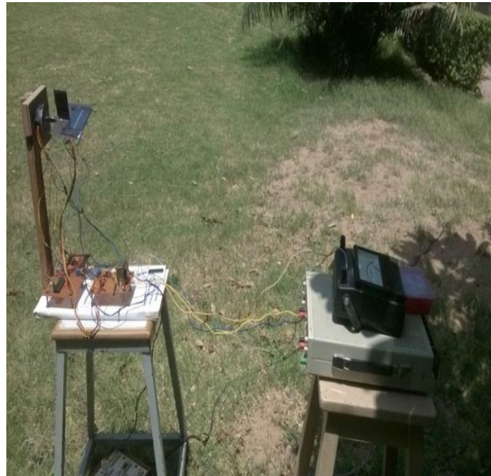
Fig. 4: Designed working Prototype of solar tracker.
